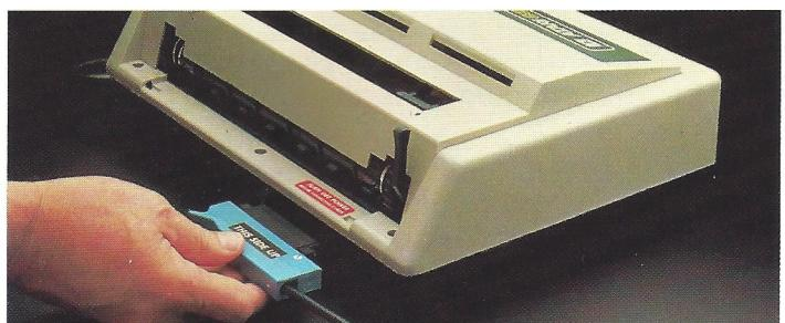
Plug a connector cable into a connector port on the front of the interface module. Plug the other end of the cable into the unused connector port on the back of the direct connect modem. Refer to the *ATARI 850 Interface Module Operator's Manual* for more detailed setup instructions. Turn on your TV.
