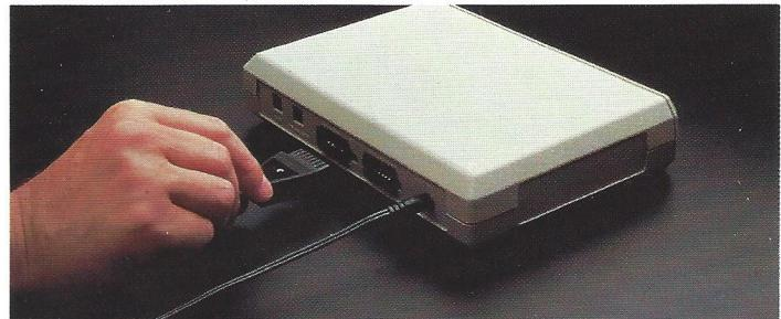
Plug the other end of the I/O cable into the connector port on the computer or other peripheral (except the **ATARI 410™ Program Recorder** or **ATARI 825™ Printer**).
